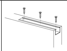
FIXER LE RAIL EN ALUMINIUM A LA PORTE AVEC LES VIS 4X30 FOURNIES. VERIFIER QUE LES VIS N'EMPECHENT PAS LE PASSAGE DE L'ETRIER.
